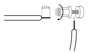
At the time make sure that the bare ends of the speaker cables do not extend from the terminals in such a way that they touch the chassis.
